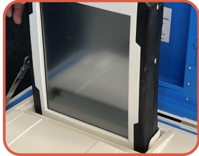
10. SEAT THE TABLET IN THE CRADLE AND TILT IT BACK.
