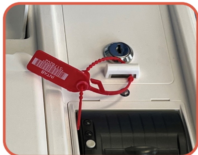
12. VERIFY THE TW RED SEAL NUMBER LOCATED ON THE VDRIVE COMPARTMENT WITH THE NUMBER ON #7 POUCH.
