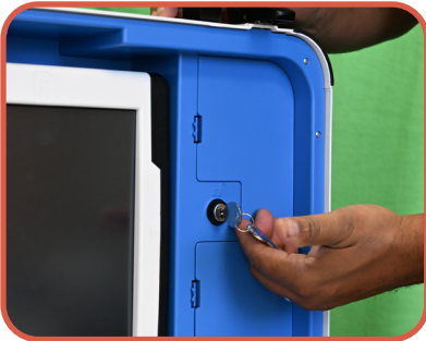
7. UNLOCK THE TABLET USING THE YELLOW/RS KEY.
