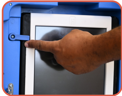
8. UNLATCH THE TABLET USING THE BLUE LEVER.
